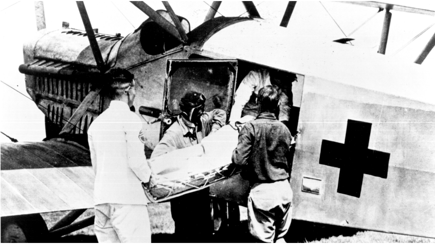
The Cox-Klemin aircraft, designed for and dedicated to aeromedical evacuation.
