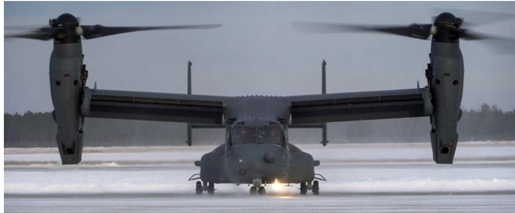
CV-22 Osprey tiltrotor aircraft, capable of vertical takeoff, landing and hover.
